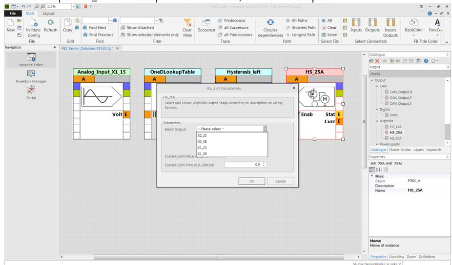
22. Connect the square angles of the function blocks by pulling lines as shown in the following screenshot.
