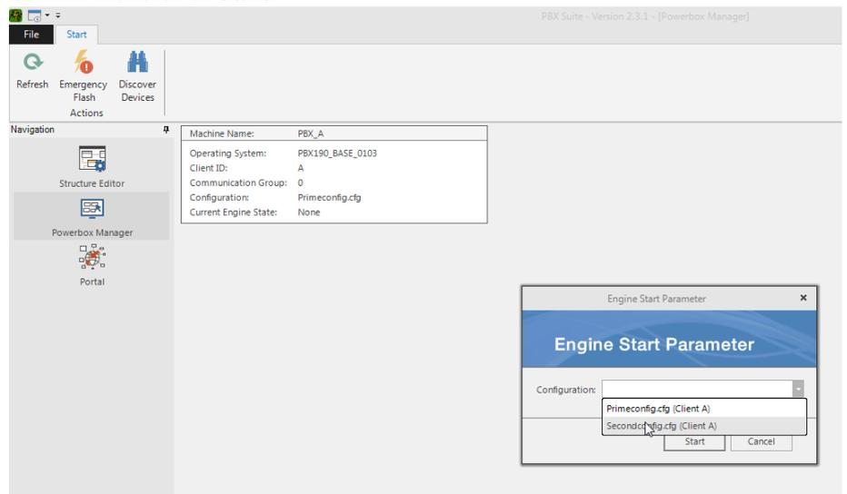
5. The device will restart, and after a short time the device window shows the name of the second configuration.
