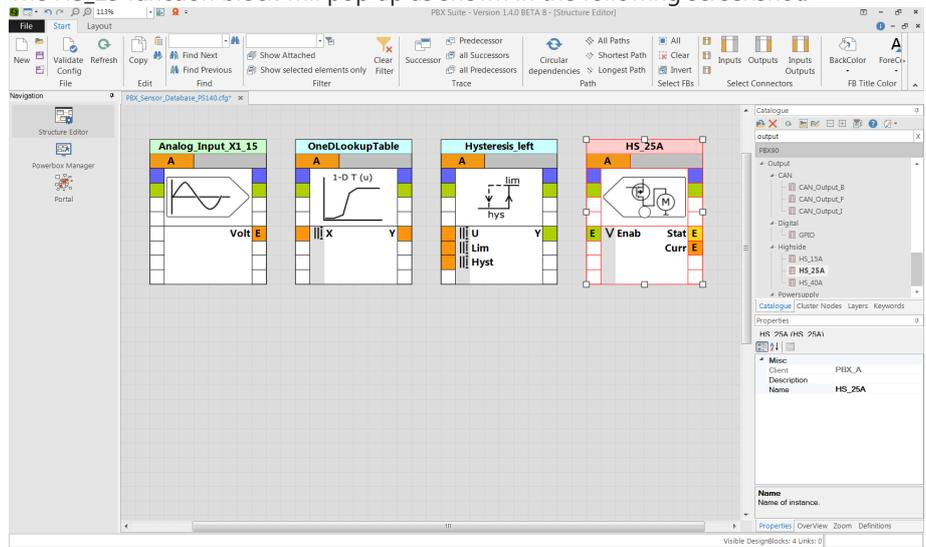
21. With double-click on the selected function block you open the pin assignment wizard. Select Output X3\_B from the pull down menu, similar to step 9.
