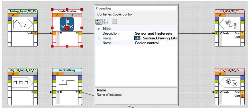
Double clicking the Container switches inside the container, showing the included functionblocks and the outside connections.
